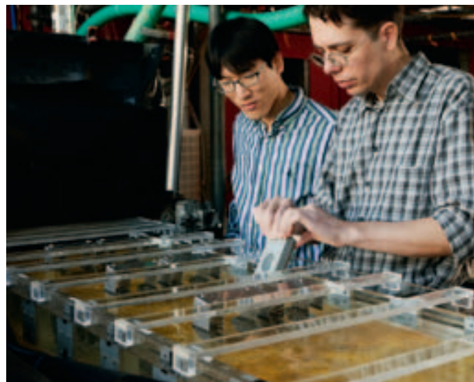
Fig. 3: In a modular flow channel experiment, Junho Jeon and Étienne Vermeirssen investigate how the sampling rate in passive samplers is affected by the membrane and environmental conditions [6].
