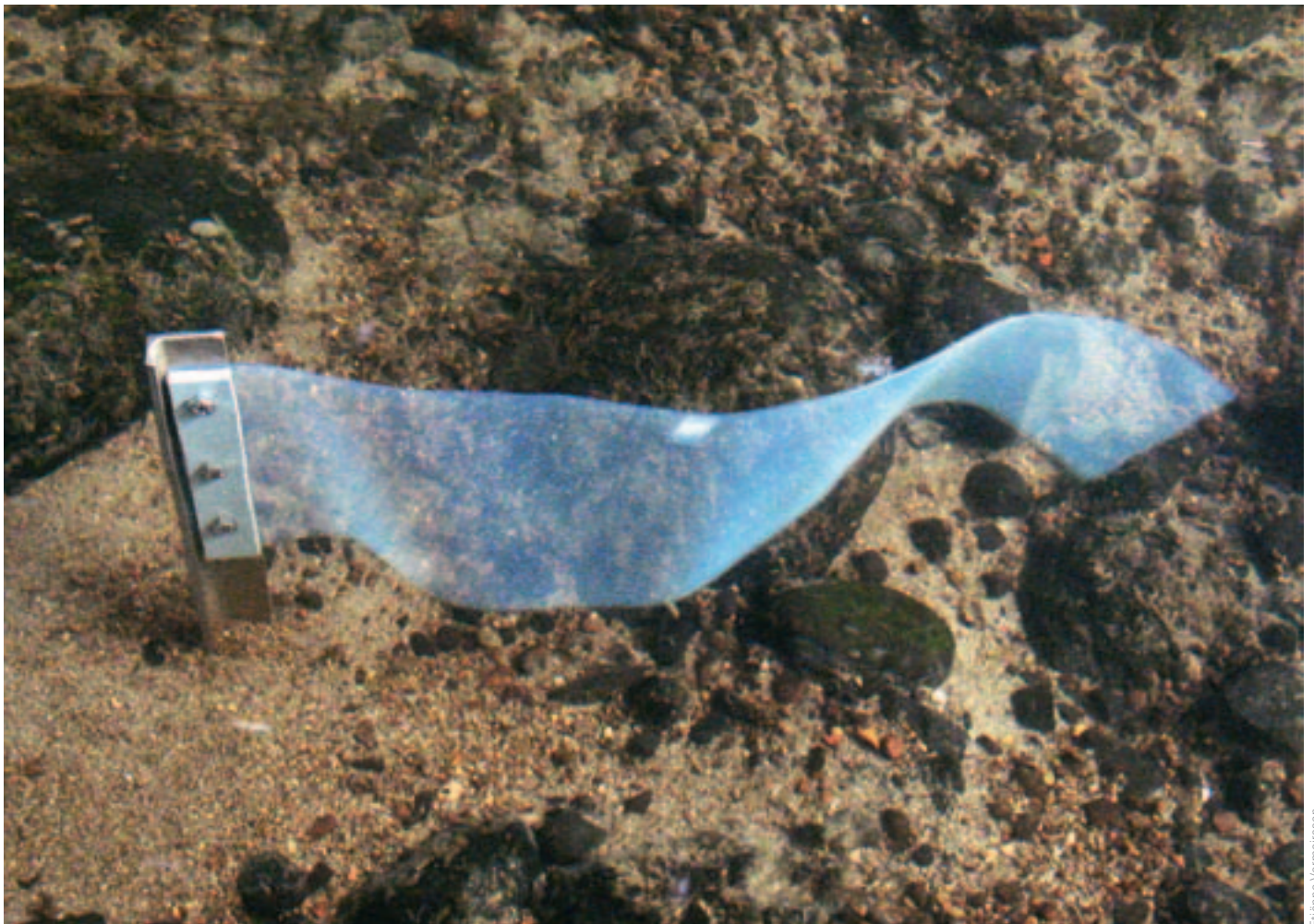
Chemicals in water diffuse into a passive sampler, accumulating in the silicone sheet.
