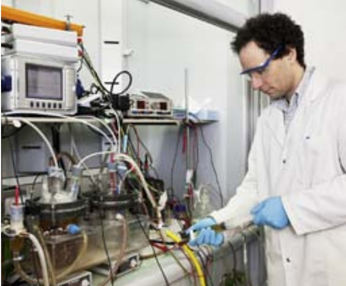
In the laboratory, process engineer Kai Udert is testing various reactors for the removal of nutrients and contaminants from urine.
