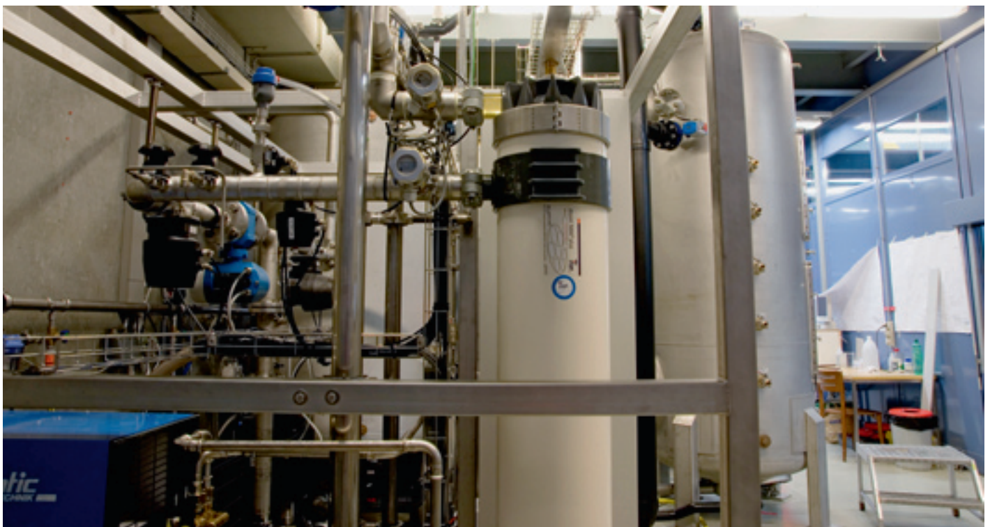
The membrane module in the pilot plant tested at the Lengg lake water facility.
