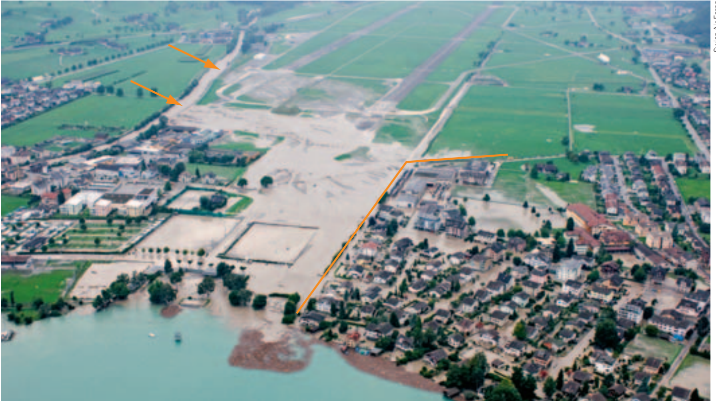
Fig. 2: The Engelberg Aa river on the plain between Ennetbürgen and Buochs during the flooding in 2005. The arrows indicate two of the three points at which the floodwaters are allowed to inundate the plain in a controlled manner. A secondary dam currently under construction is marked by an orange line.
