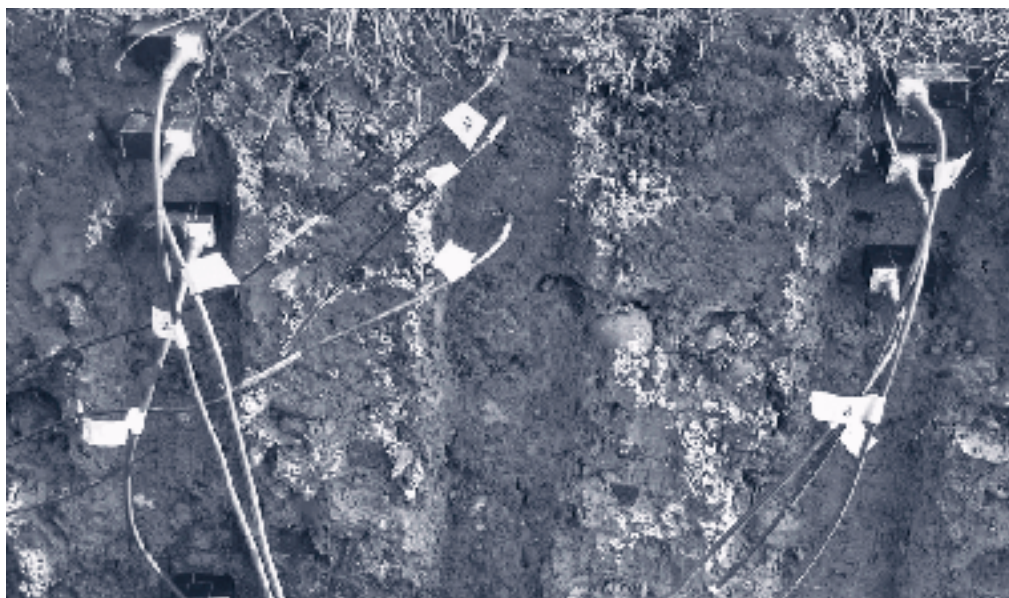
Soil profile with instruments to measure the soil water content.
