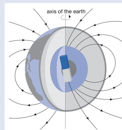
Fig. 1: The geomagnetic field can be depicted in simplified form as a dipole field produced by an imaginary bar magnet located at the earth's center. This bar magnet is slightly askew with respect to the earth's axis of rotation.
