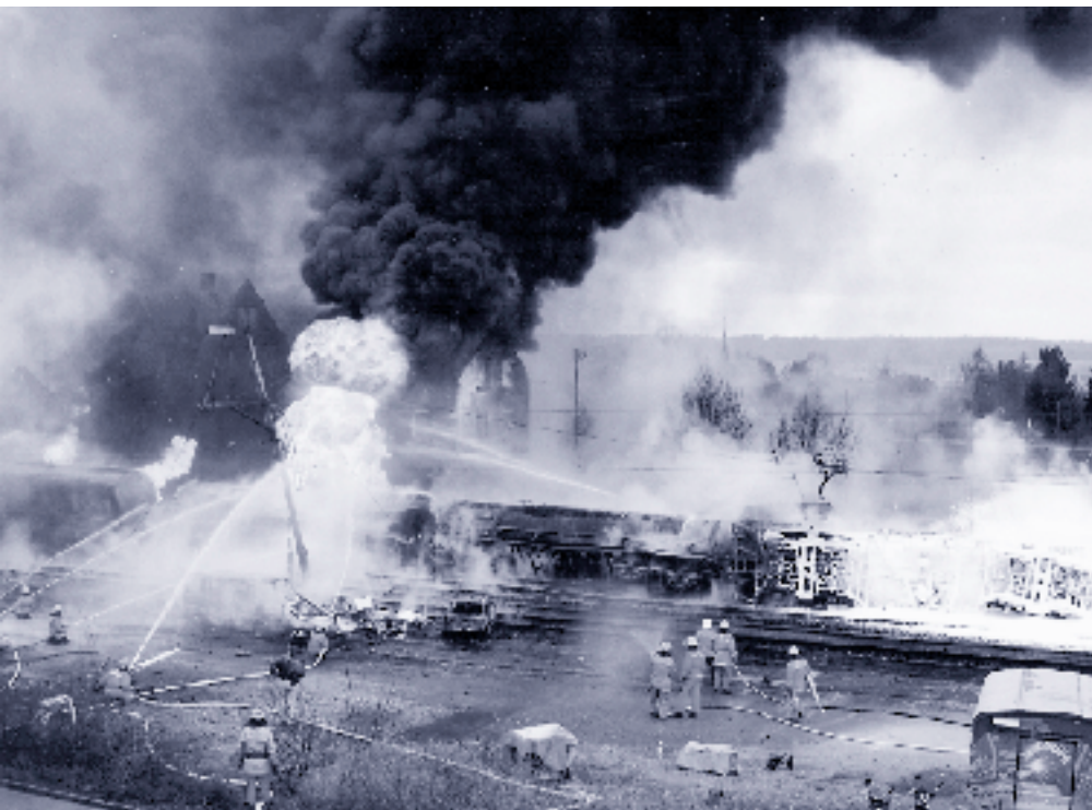
Fig. 2: After the accident of a tank train in Zurich-Affoltern in 1994, about 5 tons of MTBE reached the underground through infiltration of unburned gasoline.
